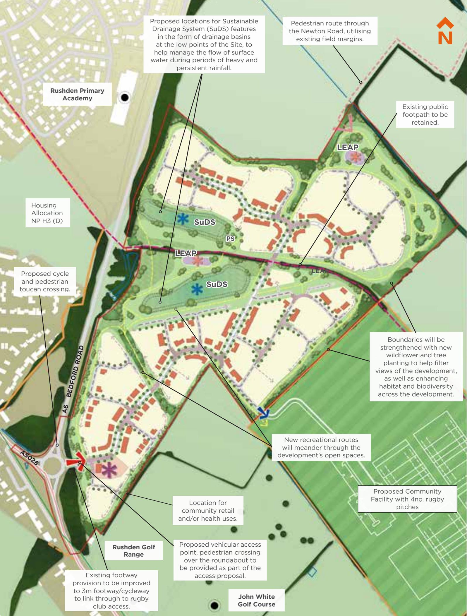
Proposed locations for Sustainable Drainage System (SuDS) features in the form of drainage basins at the low points of the Site, to help manage the flow of surface water during periods of heavy and persistent rainfall.
