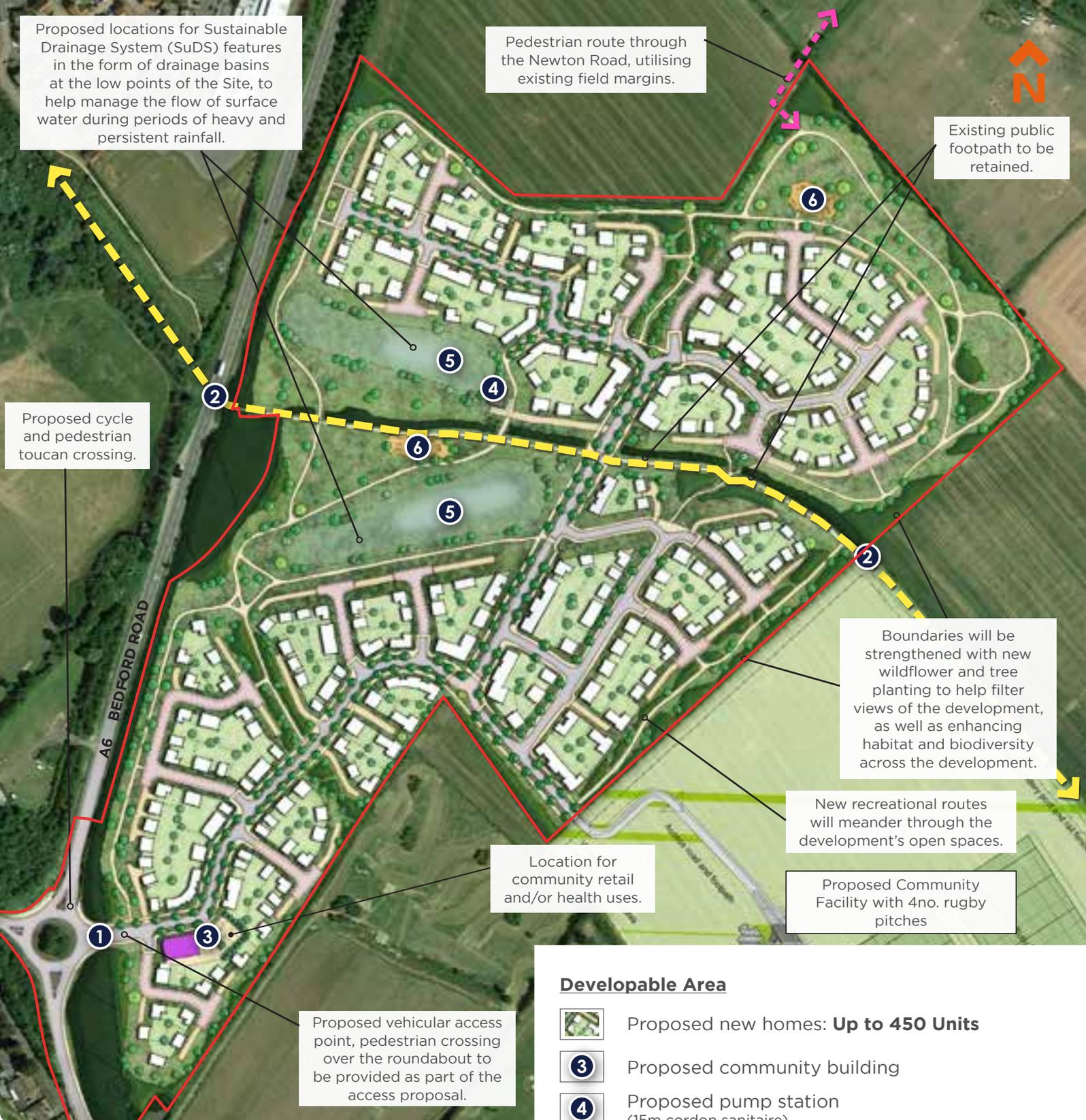
Proposed locations for Sustainable Drainage System (SuDS) features in the form of drainage basins at the low points of the Site, to help manage the flow of surface water during periods of heavy and persistent rainfall.
